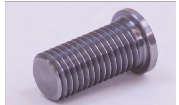
A finished piece with external threads that has been turned on a lathe.
