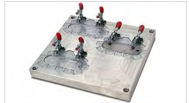
A custom fixture holds a part in place to provide consistent results each time.
