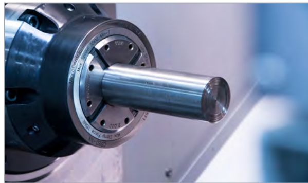
Metal rod stock is firmly fixtured in a high-speed CNC lathe before turning and milling begin.
