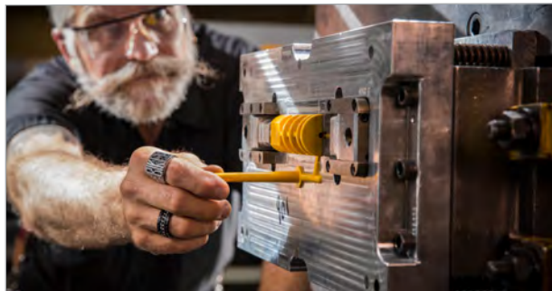
Quick-turn injection molding is regularly used for low-volume prototyping and production of plastic parts.
