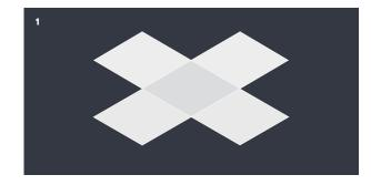
An example of flat sheet metal design is this cube without a top, which would initially look more like a plus sign. The four outer squares would be folded upward to form the sides of the open-top box.
