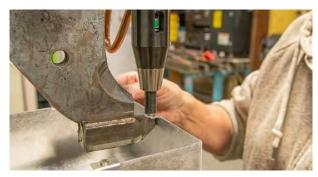
A major advantage of riveting is that your two parts don't have to be made of the same type of material.
