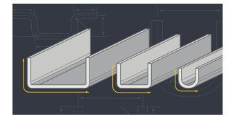
When designing U channels, consider the strength of the material you are using and how easily it can bend. Best practice is to maintain at least a 2:1 width-to-height ratio with U channels.
