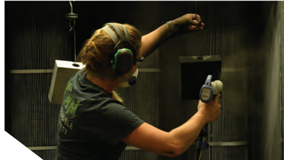
Sheet metal can be finished in several ways, including powder coating, as seen here, which results in a surface more durable than conventional paint, though it may lack paint's aesthetic qualities.
